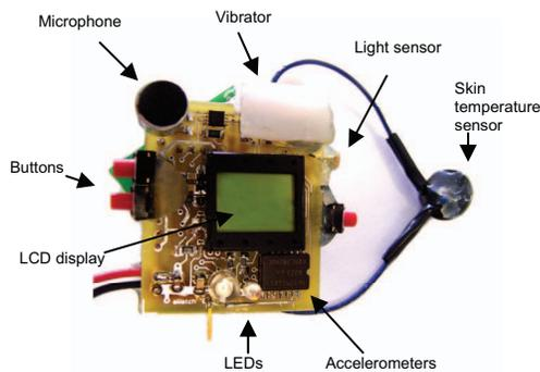
Figure 3. eWatch controller board
