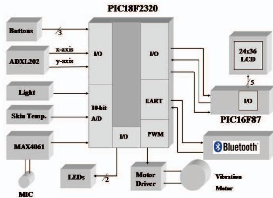
Figure 2. Hardware architecture
