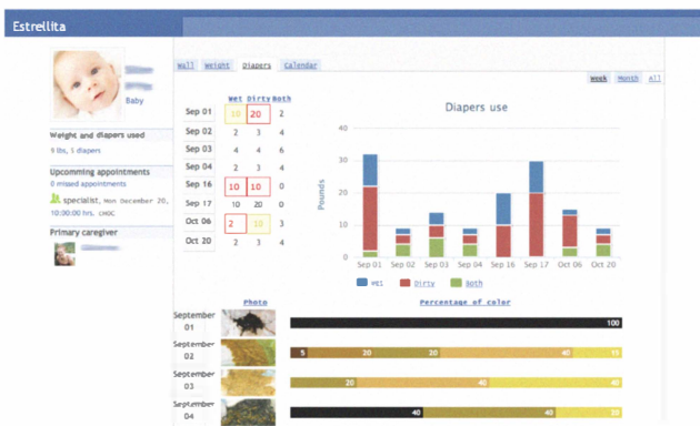
Figure 2. A screenshot of the Estrellita web portal, primarily designed for clinicians and other healthcare professionals. This particular page shows details about an infant’s diaper count, a graph of past diaper counts, and several system-generated color histograms for problematic diapers.
